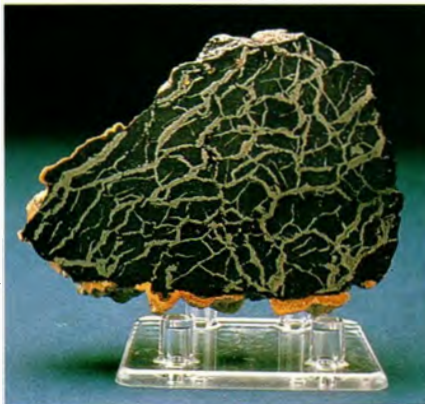
An unusual graphite nodule found near the Canyon Diablo crater in Arizona. The specimen has been etched to show a fine network of metal within the graphite. Many small diamonds have been found in this meteorite, a result of the tremendous pressure exerted on such nodules during impact.
