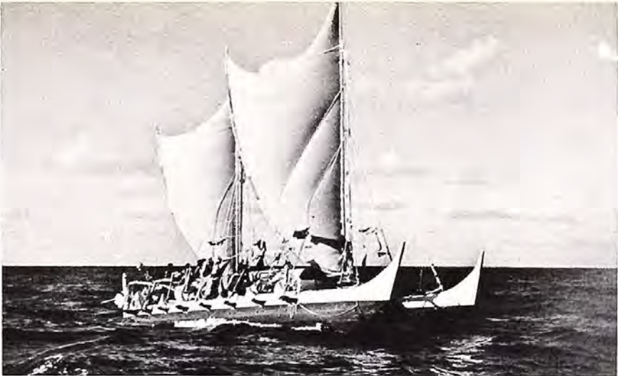
Right: The 60-foot Polynesian double canoe Hokule'a on her 2500-mile voyage from Hawaii to Tahiti; note her typically Polynesian claw-shaped sails which were reconstructed from ancient Hawaiian rock carvings.
