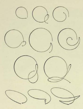
Flight tracks of a returning boomerang as recorded by Max Buchner with boomerangs specially made for testing.
